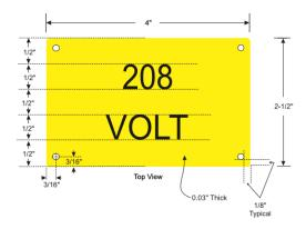
Material: 0.03" Sub-Surface Printed Velvet Textured Non-Adhesive Coated Lexan Plate, With One 1/8" Diameter Hole in Each Corner Spaced 1/8" Equally From Each Side (3/16" to center).
